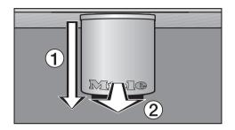
■ Pull the central spout down as far as it will go (①), and pull the cover to the spout forwards to remove it (②).
